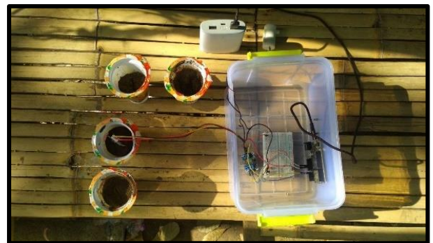
Gambar 8 Pengujian Soil Moisture Sensor
