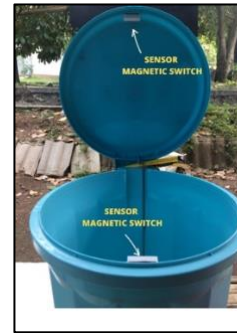
Gambar 8. Realisasi sensor magnetic switch
